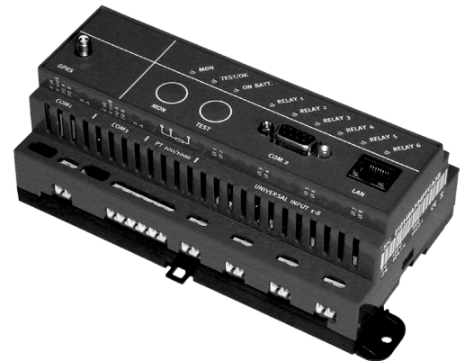
myDatalogMUC, device for the acquisition and transmission of alarms.
