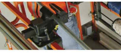
A factory-approved, rail-mounted 5  $\frac{1}{2}$  in. bench vise offers a convenient and safe method to securely hold material as you work with it—whether for threading and cutting or gripping other materials.
