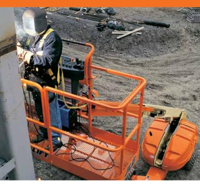
Tucked into the SkyPower<sup>®</sup> boom platform, the 280-amp Miller<sup>®</sup> CST<sup>™</sup> 280 welder conserves space and provides stick and TIG capabilities. The SkyWelder<sup>®</sup> eliminates the cost of having a stand-alone welder and power supply.
