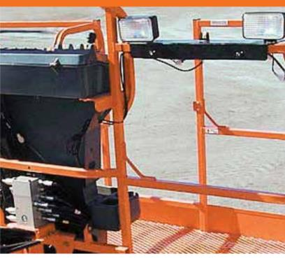
With the Nite Bright<sup>®</sup> package, you will be able to see your work environment in a whole new light. The package includes two 40-watt lights to illuminate your work site, as well as four 40-watt lights for the area around the chassis. The Nite Bright package is great for low-lit areas such as mines, tunnels and nighttime applications.
