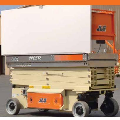
You don't need to clutter your platform with drywall, plywood or sheet rock. With the factory-approved panel carrier, you can load panels outside the rails in the carrier tray, where it's easier to transfer the panel to its elevated installation site.
