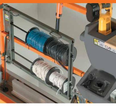
For electrical contractor applications that require batterypowered tools, the JLG Electrician's Package keeps your tools within reach and off the floor of the platform. A stowable 8 x 20 in. workbench and 6 x 6 in. molded pockets provide ample storage within easy reach for tools or fasteners while leaving the workspace open to help prevent tripping hazards.
