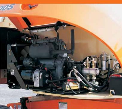
The JLG SkyPower<sup>®</sup> system delivers the power you need to conveniently operate other JLG accessories. With the SkyPower system on your machine, you get a 7500W generator with a power cable. Easily add and provide power to other JLG accessories, including SkyWelder<sup>®</sup> and SkyCutter<sup>®</sup> packages.
