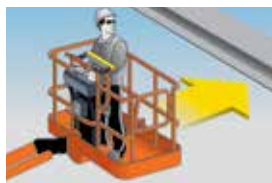
Operator moves towards obstruction.
