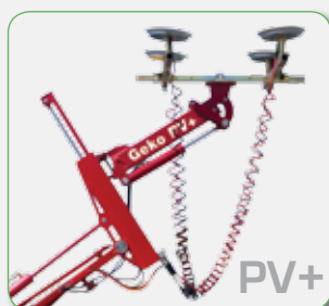
The Geko PV+ arm allows panels weighing up to 175kg to be picked up and tilted 180° for overhead and ceiling installation up to 3m high.
