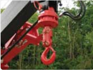
Optional hydraulic swivel hook (Capacity: 2000kg)
