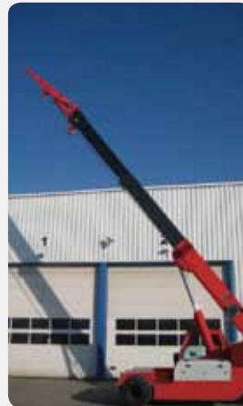
Hydraulic searcher hook (Capacity 4000kg)
