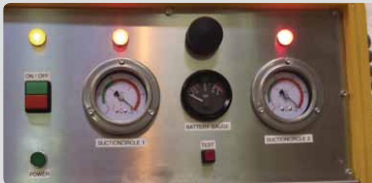
On-board control panel with vacuum and battery gauges.
