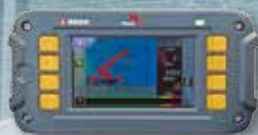
Safe load indicator
