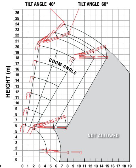
WORKING RADIUS (m) Tilt Angles 40° - 60° Outriggers extended to maximum halfway and minimum
