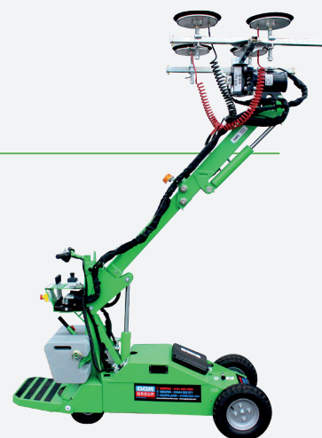
The Geko 425's platform stops movement of the robot if no operator is present.
