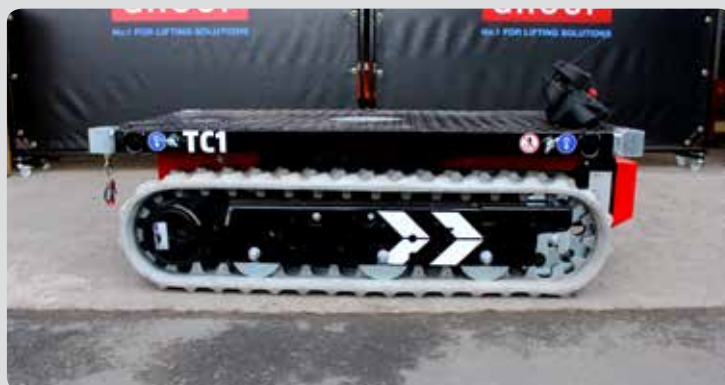
The tracks of the TC1 means it can be used to transport materials on uneven ground.
