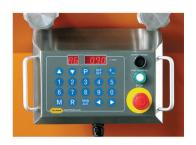
\*Digital panel can be turned off at any time with machine reverting to a single angle preset system If the panel fails or is unneccesary for the job, you can still bend with full control and accuracy.
