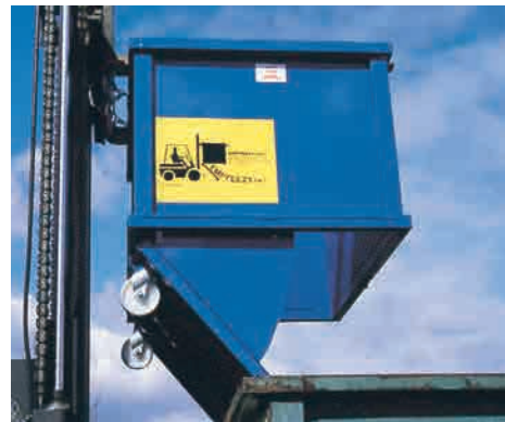
CHUTE MOUTH - FLANKED BASE TO AVOID SIDE SPILLS
