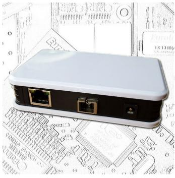
**ONU-1GE** fully comply with IEEE 802.3-2005. It is operative, manageable and maintainable at telecommunication level, and can provide high speed data service for customers. It has a PON uplink port that connects to office end apparatus through optical fiber.
