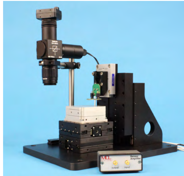
▲ AFM with motorized XYZ approach, video optical microscope, and coaxial illuminator
