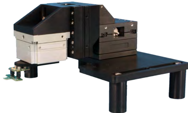
▲ Three axis probe positioner with three axis micropositioning of the probe head. Ideal for use on optical tables when mounted on an optional platform (as shown). The probe nanopositioner is a compact custom nanopositioner with 100 \times 100 \times 20 \mu\text{m} of travel. The probe head micropositioning is the MMP3H micropositioning system.
