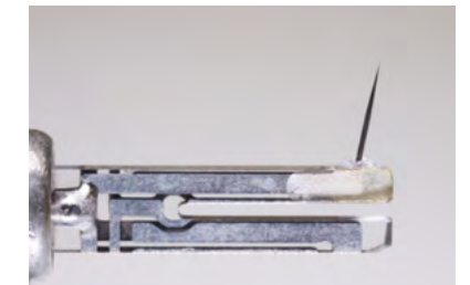
Tuning Fork with etched tungsten tip
