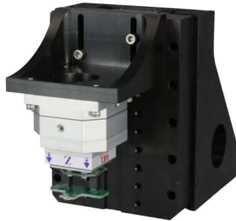
▲ A three axis high resolution tip scanner. A single axis motorized approach is provided by the SPM-MZ. The high resolution tip scanner is the Nano-HS3M with 10 \times 10 \times 5 \mu\text{m} of motion. This example is designed for users who require picometer precision.
