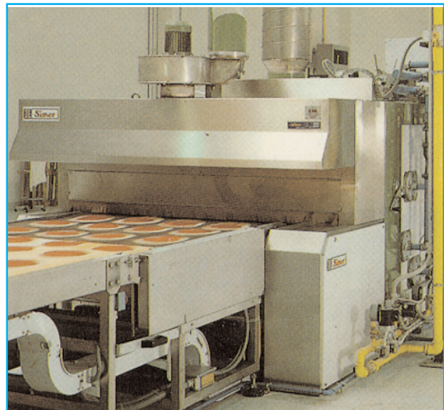
Pizza baking oven with direct flame burners, model Ribbon (Simer)
