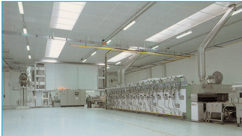
Pizza baking oven with direct flame burners, model Ribbon (Simer)
