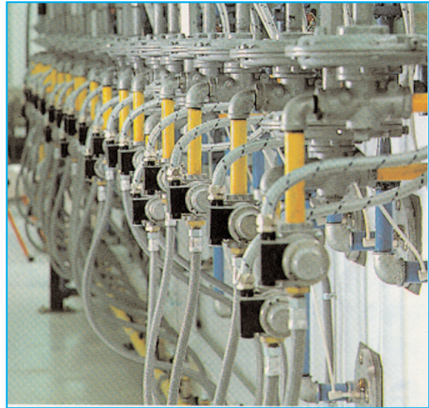
Pizza baking oven with direct flame burners, Flomixer (Simer)
