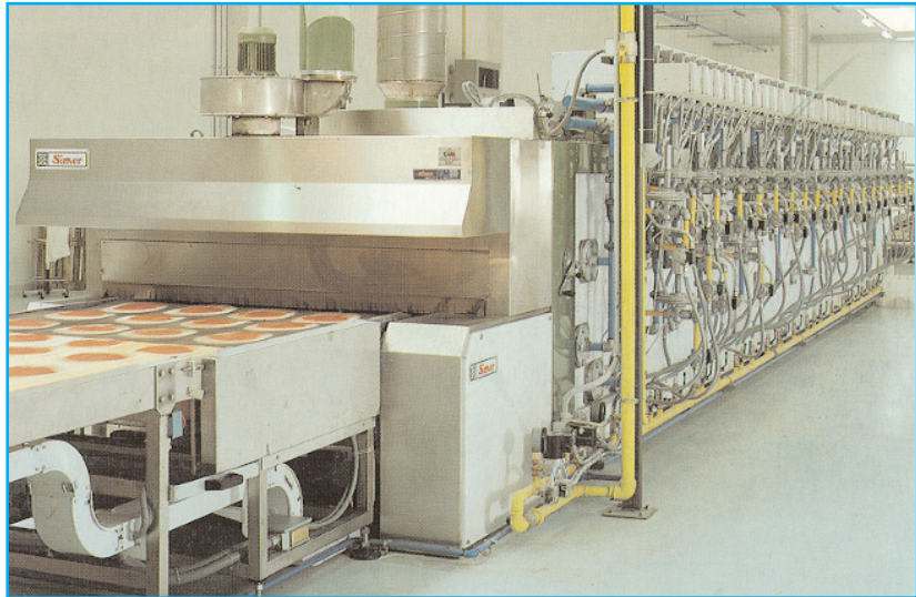
Pizza baking oven with direct flame burners, model Ribbon (Simer)
