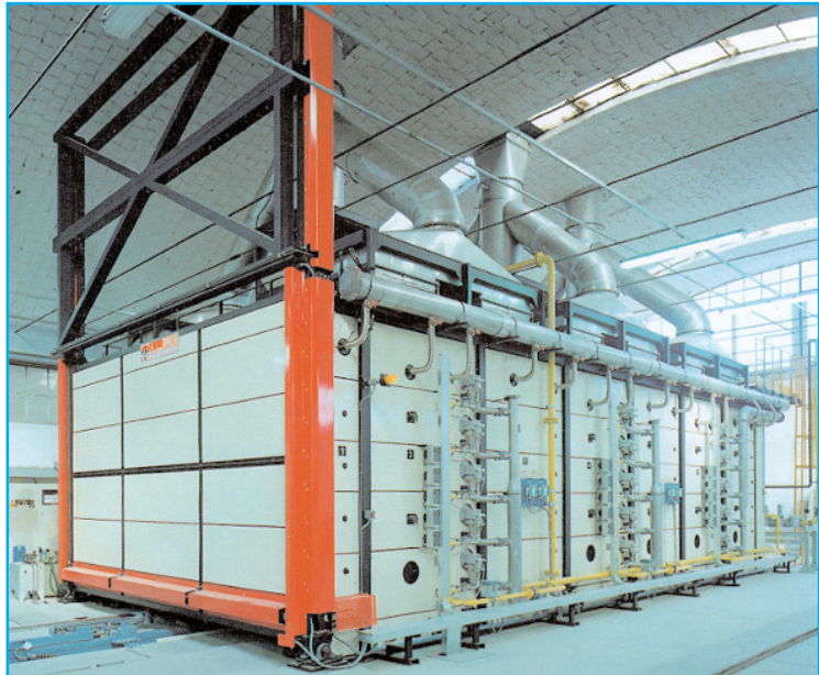
Sanitary fittings baking furnace with burners, model EMB-3-SIK, electronic reducing regulator (Poppi Eurotech)
