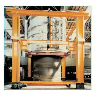
Combustion plant with highspeed, recuperative burners.
