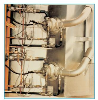
Combustion plant with highspeed, recuperative burners; application on cone furnace
