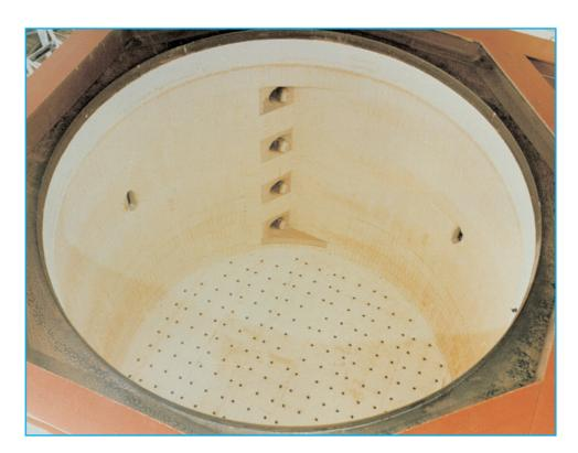
Combustion plant with high speed, recuperative burners. Application on cone furnace
