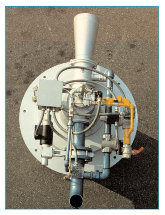
High speed, recuperative, pre-assembled burner group equipped with air and gas pipes, pilot burner, exhaust manifold, electrical wiring, pull box, block holder with metallic protection (CIB)
