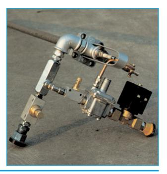
Detail of pilot burner for recuperative burners (CIB)
