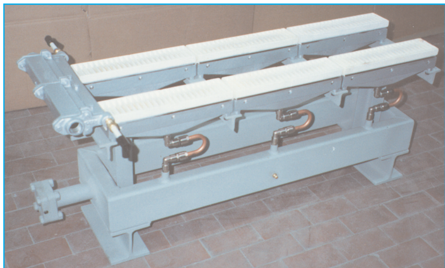
Radiant panel with burners IRC-1 for crêpes baking (Unilever Italia Sagit)
