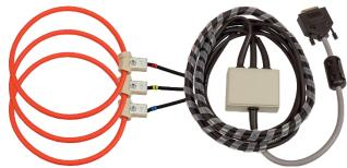
Flexible current clamps (Rogowski coils) FCT3000AC allow for easy current measurement on cables and bars in electric installation. Due flexibility and small sensor diameter it is easy to assembly them in hard access places. Maximum diameter of cable, on which we can close the sensor is about 150mm.
