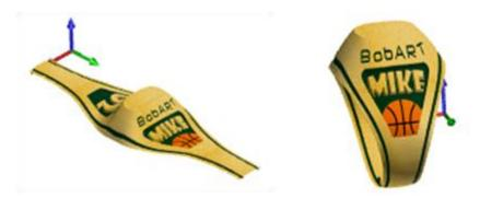
With the Remove Non-Emboss Area option, now you decide what to include in the model. You can save the model with or without the non-embossed areas (when using Save Whole Emboss as Component/STL or Save Whole Emboss to BobART Surface File).
