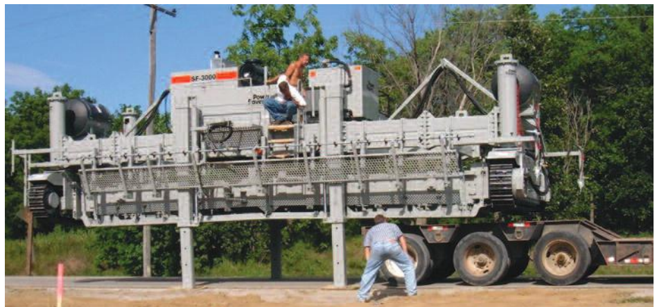
Hydraulic loading legs lift the entire machine allowing the trailer to back underneath. Quickly move the machine from job to job.
