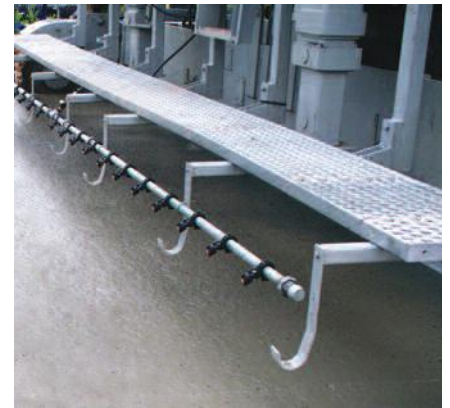
Hooks for a burlap drag and an optional water misting system enhance finishing choices.
