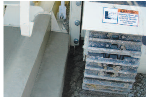
An optional curb mold, even for specialized profiles, can add integral curb to one or both sides of the pavement.
