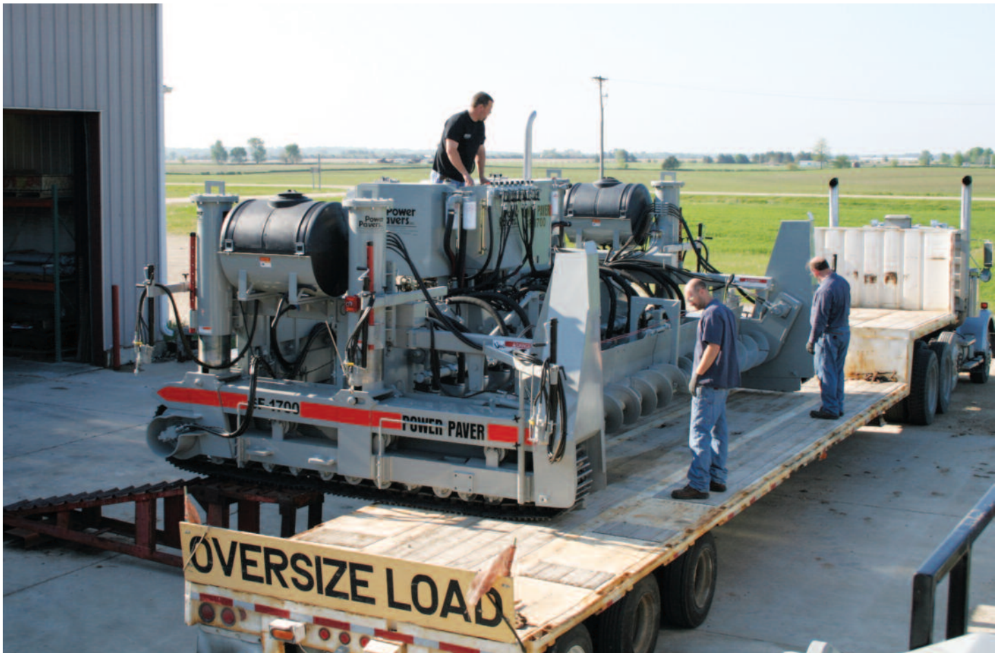
Loading and unloading the SF-1700 and SF-2700 pavers is quick and easy with side ramps.
