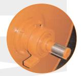
A cast iron trunnion and pillow block house a triple seal protection system utilizing both rigid steel washers and flexible synthetic grease seals. This system provides for protection from contamination and premature failure.
