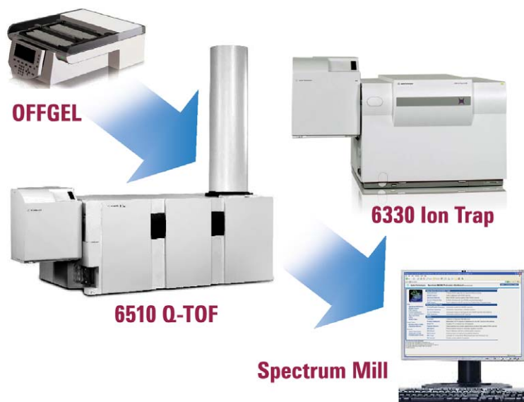
Figure 1. The experimental workflow consisting of a 3100 OFFGEL Fractionator, a 1200 HPLC-Chip/6510 Q-TOF LC/MS, and Spectrum Mill software for data analysis. As part of this study, the performance of the Q-TOF was compared with the 6330 Ion Trap mass spectrometer.
