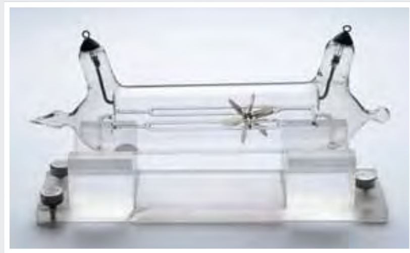
Bottom right: Crookes Tube, an evacuated glass tube with 3 node elements (one anode and two cathodes). Late 1800's.
