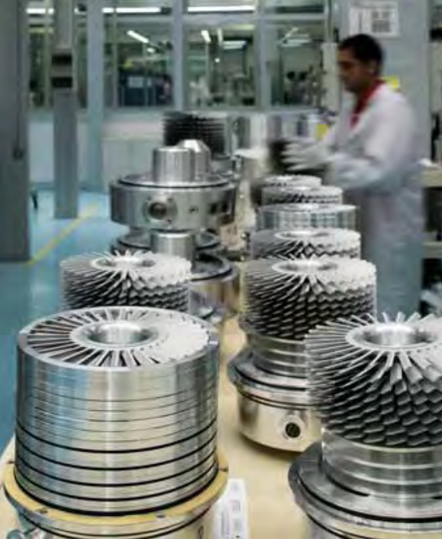
Left: Large Turbo Pump rotor/stators assembling. Patented MacroTorr® Stages (visible on the pump in close-up) technology greatly improved pump performance.
