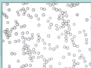
Figure 1. Magnified image analysis was used to compare SPE polymer particle sizes
