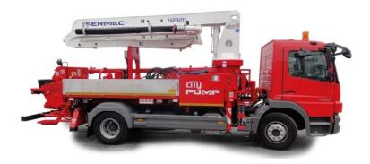
The concrete pump **4ZR20** has been specifically designed for operate small jobsites and covered places. The pump is equipped with a **4-sections boom** that can be opened in **4,2 meters only**. The pump is comfortable in any city centers thanks to the mounting on compact **2-axles** truck (**wheelbase 3.650-4.000 mm**); typical applications are renewal works, service structures, city roads & up to midsize pave ways.
