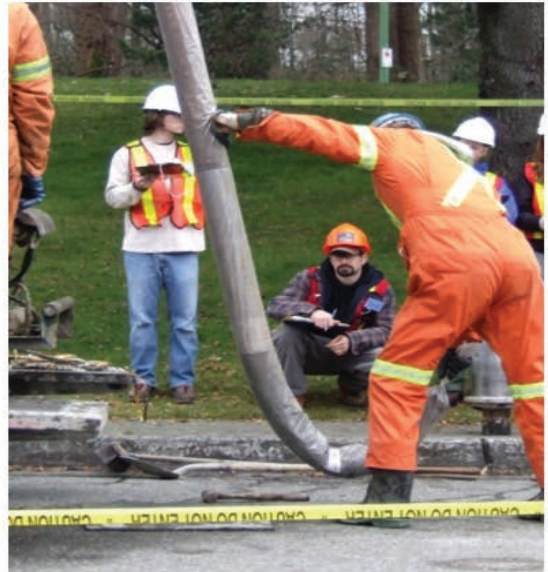
A SAMPLE BEING EXTRUDED INTO PLASTIC CORE BAG
