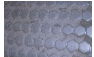
Built-up autogenous wear-protection layer
