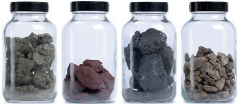
Test work materials for grinding: cement clinker, iron ore, blue lead, diamond ore
