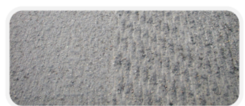
.47" (12mm) 2R 2 Fine Mill Drum vs. .31" (8mm) Triple Wrap Drum at same cutting speed
