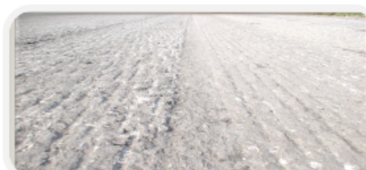
.31" (8mm) Triple Wrap Fine Mill Drum (300 tools) vs. 2R 2 Standard Drum (200 tools)
