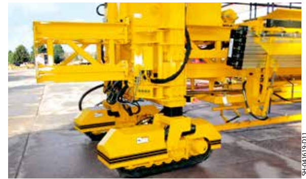
The walking end car allows the T/C-5600 to turn its tracks and walk the end car in or out for additional end sections to be added or removed.
