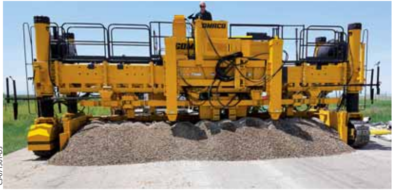
The GOMACO PS-2600 with the 7500 series placer mold is placing rock. The placer's auger has a diameter of 24 inches (7.32 mm).
