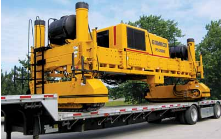
The GOMACO PS-2600 has a minimum transport width of 12 feet (3.66 m) and a transport height of 9.75 feet (2.97 m) without the strike-off mold. The PS-2600 also has a minimum transport length of 19 feet (5.97 m) with the 12 foot (3.66 m) strike-off mold attached.
