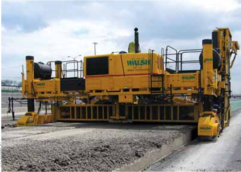
The unique telescoping frame extends 6.5 feet (1.98 m) on the left side of the frame to accommodate variable-width applications.
