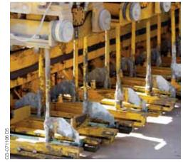
**2:** The forks wait in stand-by mode for the insertion point to be signaled by the G+ control system. The bar loading trays have adjustable-height bar extractors and the trays have been designed for easy bar spacing and width changes to meet each project's exacting specifications.
