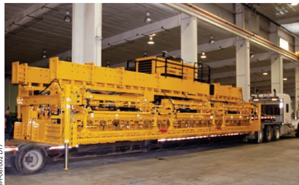
The IDBI attachment has outriggers, capable of supporting its full weight, for attaching or detaching from the paver, or raising for transport on a trailer.
