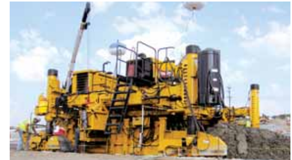
A Commander III with IDBI attachment slipforms 12 feet (3.7 m) wide on a project in Marietta, Ohio.
