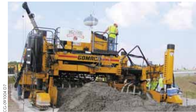
The four-track Commander III and IDBI attachment is capable of paving widths up to 16 feet (4.9 m).
