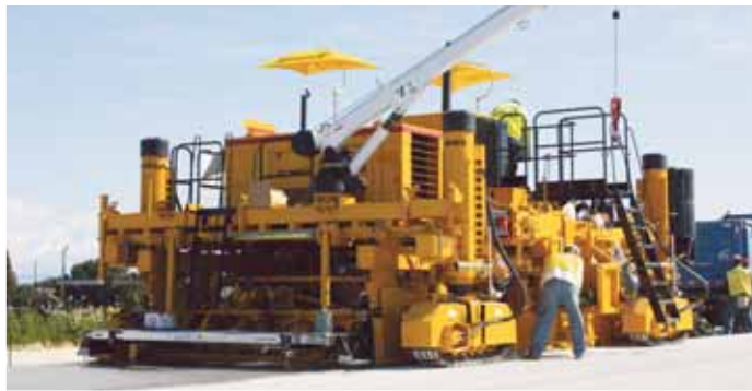
The IDBI attachment is an independent unit from the Commander III and is powered by its own engine.
