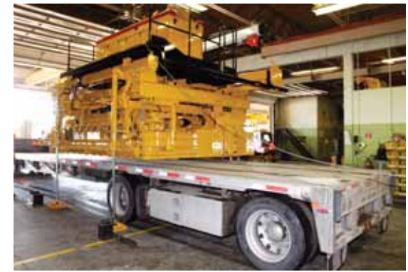
The IDBI attachment has outriggers, capable of supporting its full weight, for attaching or detaching from the paver, or raising for transport on a trailer.
