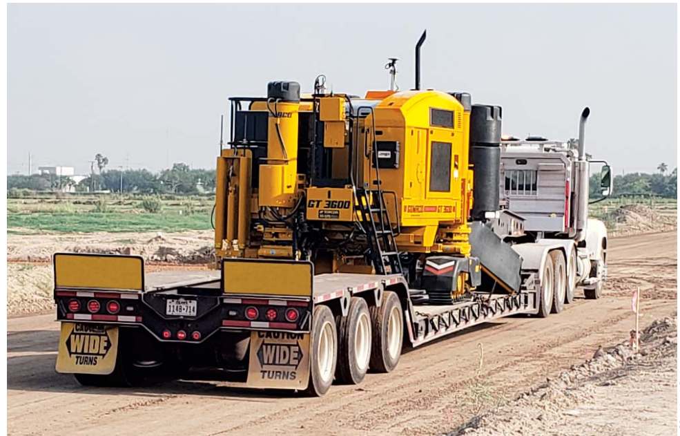
Designed for easy transportation, the Xtreme GT-3600 curb and gutter machine can be driven straight onto the truck bed after a day of slipforming.
