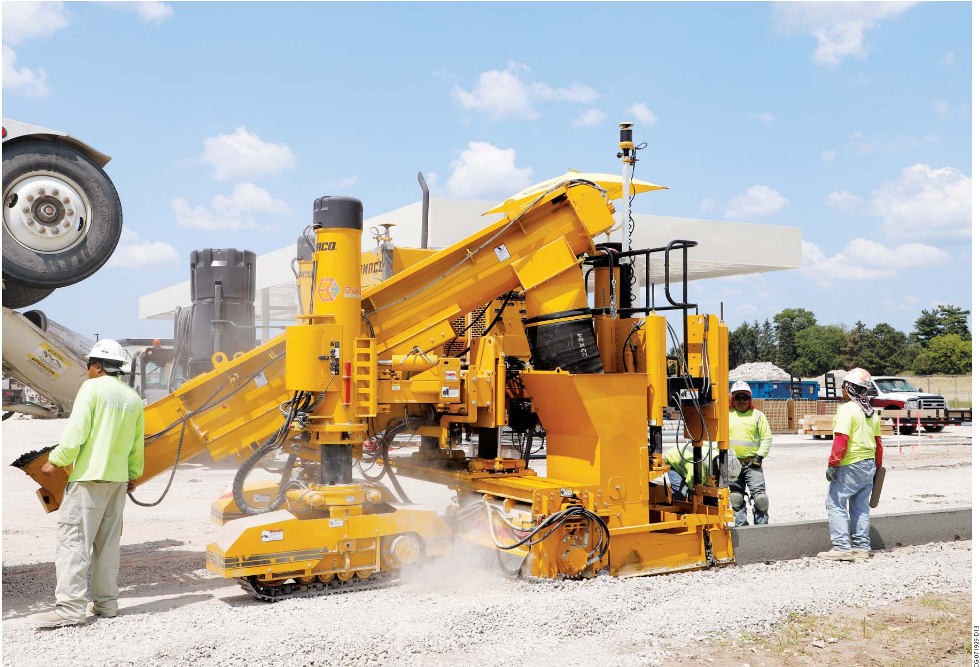
The powerful trimmerhead features a direct drive radial piston hydraulic motor that provides maximum torque for tough trimming applications.
