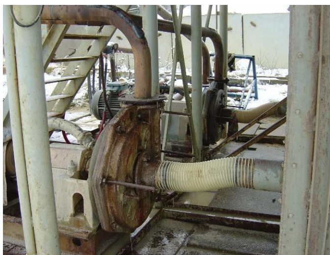
MAPE 100, Transportation of wet sand during separation into fractions
