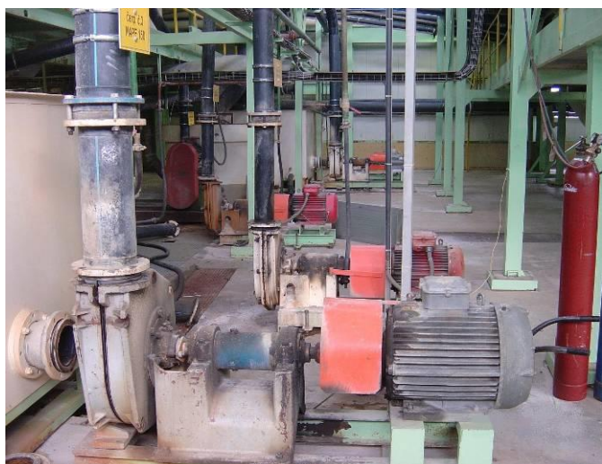
6x MAPE 150, Treatment and washing process of silicium sand
