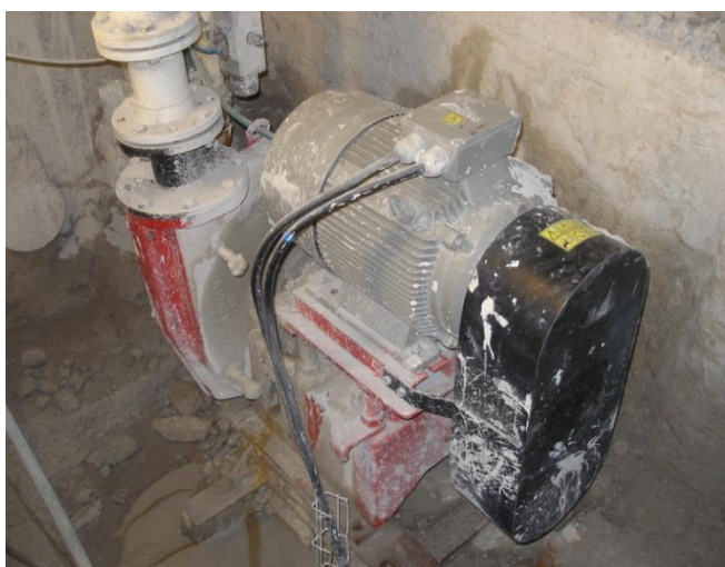
MAPE 100, Transportation of the concrete during the production of gas-silicate blocks
