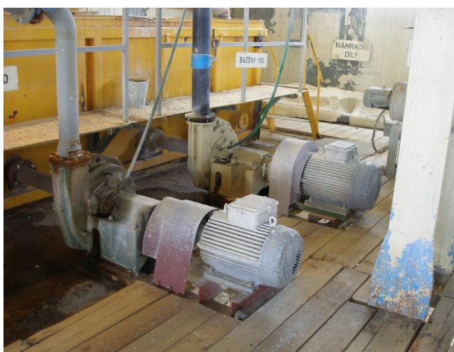
2 x MAPE 100 Transportation of water during kaolin washing
