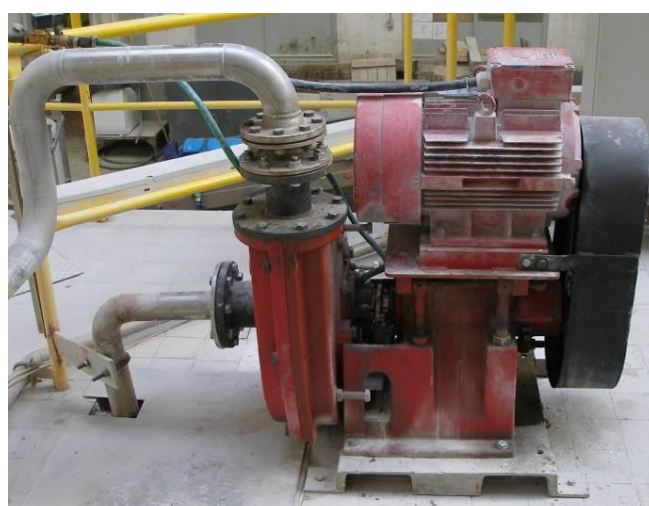
MAPE 100, Transportation of ceramic slurry into a pressing machine
