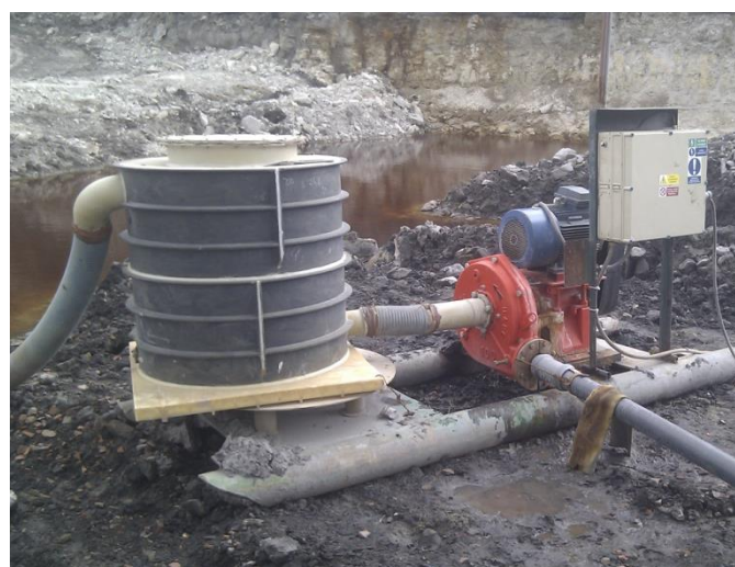
MAPE 100 Transportation of mine water during the extraction of ceramic substance. Installation of countershaft tank
