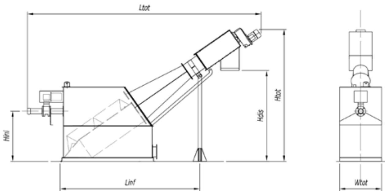
**Impianti compatti di trattamento bottini modello 05-0364 / Compact system for sewage trucks acceptance model 05-0364**
