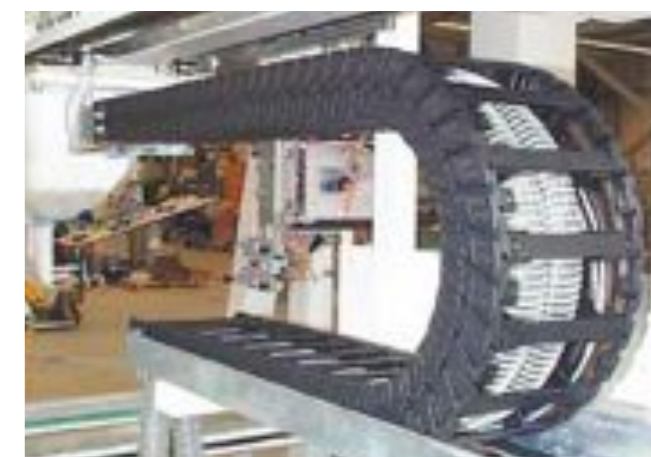
System E6 in einem CD-Hüllen-Entnahmeroboter System E6 in a pick and place robot for injection molded CD covers
