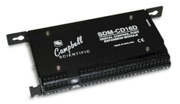
The SDM-CD16D is intended for low voltage, low power applications not suitable for the SDM-CD16AC. The unit cost is also considerably lower.
