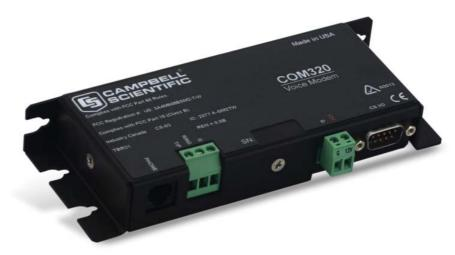
The datalogger connects with the CS I/O port on the COM320 via an SC12 or SC12R-6 cable. The RJ-11C jack is for attaching a surge-protected telephone line. Alternatively, the screw terminals (GND, RING, TIP) can be used to connect the COM320 with a phone line via a surge protector.
