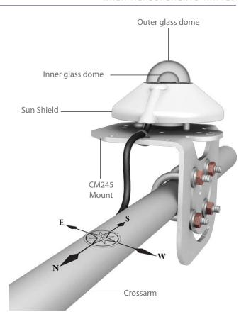
These pyranometers include a white sun shield that reduces the sensor's temperature. The bubble level is viewable while the sun shield is attached. The pyranometer is typically mounted and leveled horizontally.
