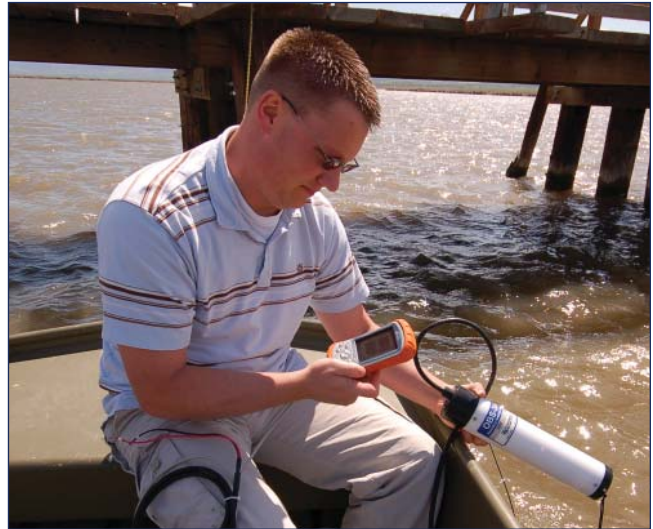
The Archer-OBS (center) can be easily carried to a lake, river, pond—anywhere an OBS-3A (right) is making measurements.
