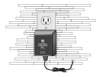
One end of the #9591 transformer plugs into a wall ac outlet while the other end connects to the PS100 Power Supply.
