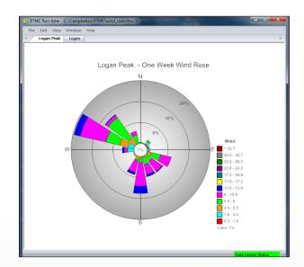
With RTMC Pro, users can create a wind rose report that displays the distribution of wind directions at various wind speeds.
