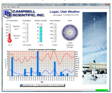
RTMC projects developed in RTMC Development or RTMC Pro are run using RTMC Run-Time. RTMC Run-Time is included with LoggerNet, LoggerNetAdmin, RTDAQ, and RTMC Pro. Additional RTMC Run-Time versions can be purchased separately and installed on computers that are networked to a LoggerNet computer. This allows remote computers to display data in a graphical format from a LoggerNet server.
