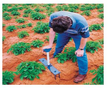
Specialized tools and techniques offered by Campbell Scientific simplify probe installation while minimizing soil disturbance. The EasyAG II (shown here) can be installed in soils ranging from light sand to heavy clay.
