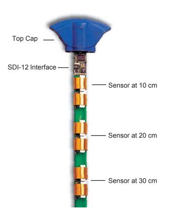
The EasyAG II probe is ideal for measuring soil water content profiles in agricultural soils.
