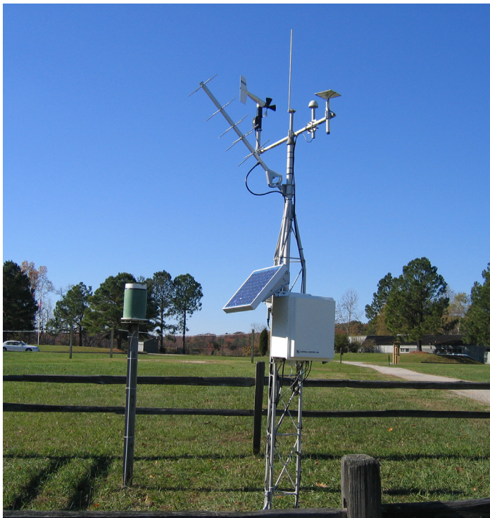
This station for the National Estuarine Research Reserve (NERR) in Virginia transmits data using a satellite transmitter.
