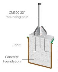
A cut away view shows a 23" pole attached to a concrete foundation via j-bolts. Order a CM300-PJ to get a 23" pole with the J-bolt pedestal kit.
