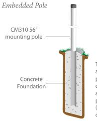
This cut away view shows a 56" mounting pole placed directly in a concrete foundation. Order a CM310-NP to get a 56" pole with no pedestal kit (see Ordering Information on page 2).
