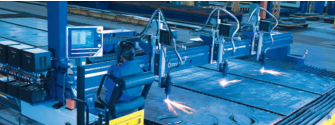
The gantry machine OmniMat® – here with three plasma torches – offers high cutting accuracy and faithful shape following in 24 hour continuous operation.
